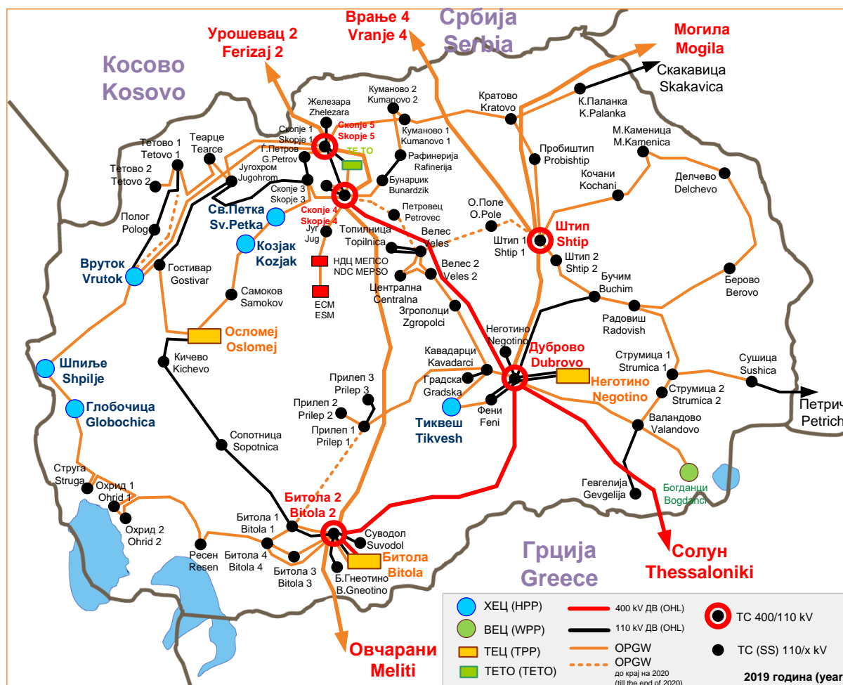
Figure 3. OPGW ground wire cross transmission lines in the transmission network
